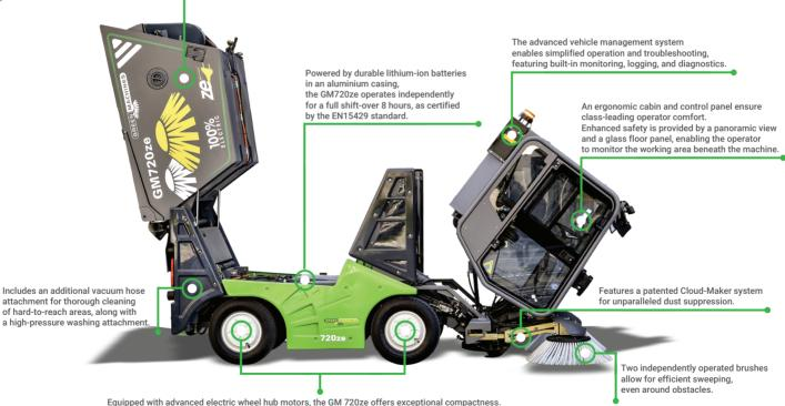
Equipped with advanced electric wheel hub motors, the GM 7202e offers exceptional compactness. Its four-wheel steering dramatically reduces the turning radius, making it ideal for tight urban environments.
