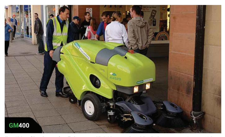
Clean with the confidence that comes from effortless maneuverability in tight spaces and around obstacles. Sweep smarter, covering more area in less time due to reduced dump cycles by compacting waste down to 33% of its original size. The optional Wanderhose allows cleaning in extremely tight spaces. Just ten litres of fuel/day gives 10 hours' sweeping time.
