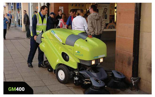
Clean with the confidence that comes from effortless maneuverability in tight spaces and around obstacles. Sweep smarter, covering more area in less time due to reduced dump cycles by compacting waste down to 33% of its original size. The optional Wanderhose allows cleaning in extremely tight spaces. Just ten litres of fuel/day gives 10 hours' sweeping time.
