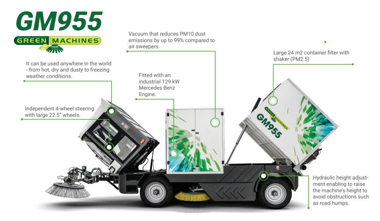
The tilting cabin is suspended by shock absorbers granting swift access to the engine and hydraulic systems so maintenance can be performed with ease and high efficiency, saving time and money.
